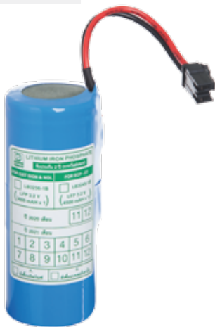
Model: EXTA36-1B Nominal voltage: 3.2 V Nominal capacity: 3600 mAh For DYNO exit light model: XLF-S10N/R, XLF-S15N/R, BXF-10N/R, TSF-10N
