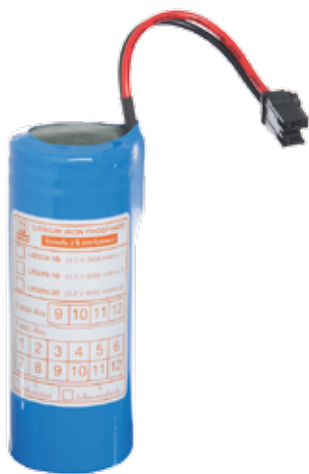
Model: ED3236-1B Nominal voltage: 3.2 V Nominal capacity: 3600 mAh For DYNO emergency light model: EPD-209
