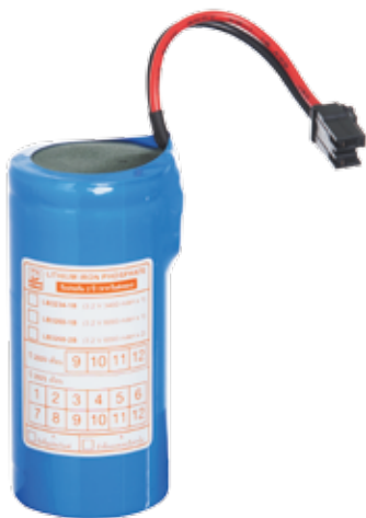
Model: LB3260-1B Nominal voltage: 3.2 V Nominal capacity: 6000 mAh For DYNO emergency light model: LFG-09P3T, ECP-2T, RES-09P3T
